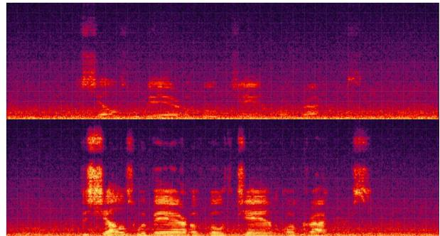
Fig. 2.: Spectrograms of the driver signal recorded at the rear passenger's ear in the 3<sup>rd</sup> row. Top: ICC off, bottom: ICC on
